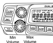
**NOTE** Hold ,keep pressing it to Monitor the background noise after the transceiver emits a DU beep, meanwhile adjust the [VOLUME] knob. During communication, volume can be adjusted more accurate.
