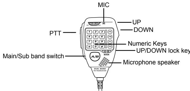
You can operate the transceiver by keypad or input desired frequency and channel through the QHM-05 microphone.
